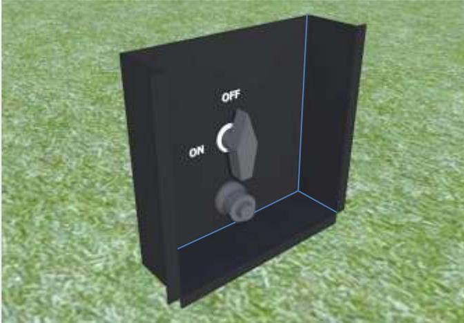
2. Install the igniter by unscrewing the top cap and hex nut counter-clockwise. Once the top cap and nut are separate, place the box portion on the inside of the unit with the threaded body through the hole. Insert one AAA battery positive end outward. Hand tighten the nut and cap to complete the assembly.
